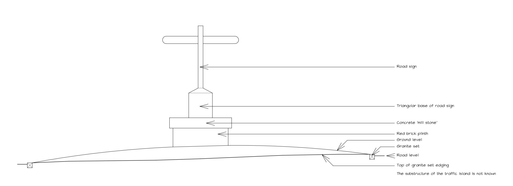
EXISTING ELEVATION The traffic island is shown tyransparent to indicate details
